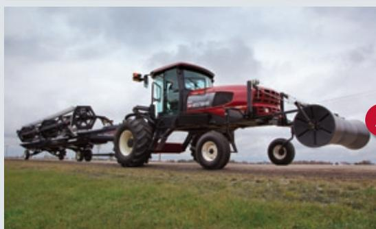
**5** *Attach hitch to weight box, rotate operator station from field to highway mode*
