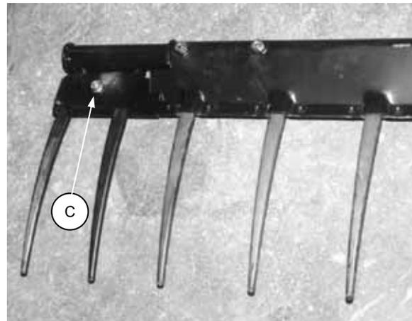
LOOSEN BOLT TO REMOVE
