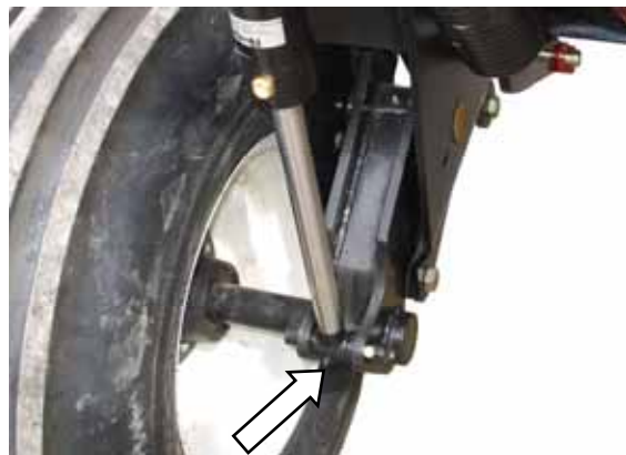
CYLINDER PIVOT 1 PLC
