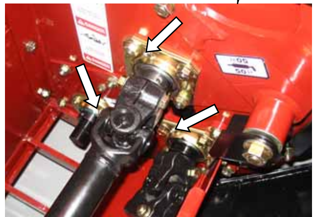
ROLL SHAFT BEARINGS (3 PLCS)
