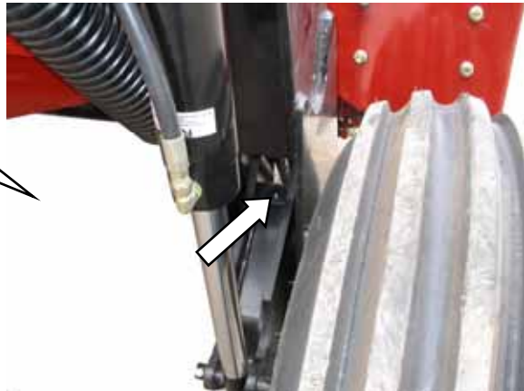
LIFT LINK 1PLC – BOTH SIDES
